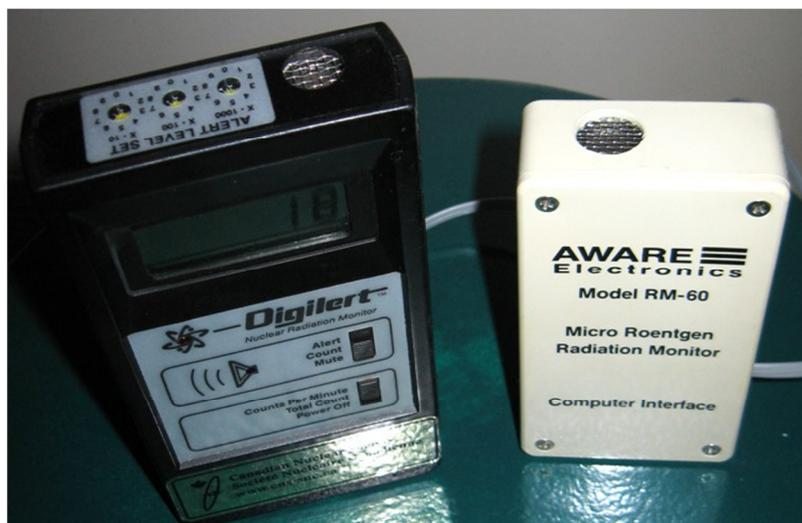
The RM-60 is compared with the larger RM-80 in the table below. The area ratio is 23.6 while the sensitivity ratio is 3.24 (neglecting any effect of the differences in energy of the reference nuclide gamma emissions).
