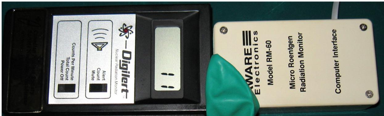
The RM-60 count rate rose to 231 counts per minute while the Digilert count rate rose to 149 counts per minute – over 10 X background. Inserting a piece of paper reduced the count rate for the RM-60 but did not seem to have as large an effect on the Digilert. Moving the Geigers and the balloon changes the count rate. To test this further the balloon was folded to provide 8 layers over the window area. This increased the count rate to 340 CPM for the RM-60 and 245 for the Digilert.
