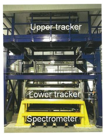
Figure 2: CRIPT tracking layout.
