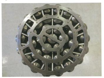
**Figure 8:** Mock fuel bundle - cross sectional view. Note: The central element was removed from the bundle referenced in this paper.
