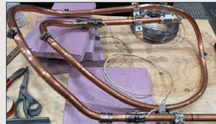
Non-planar stellarator HTS coil prototype from Type One, MIT, CFS collaboration
