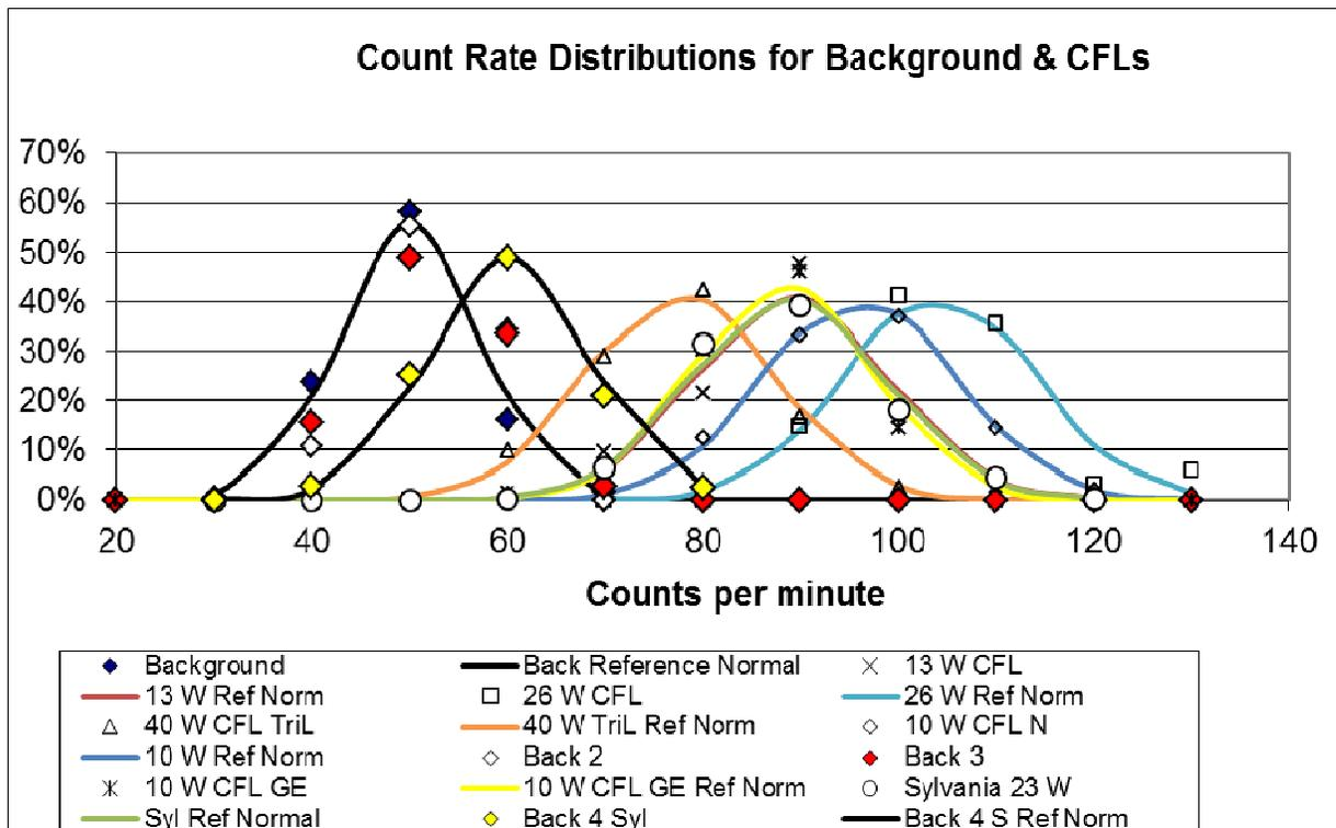
Histograms of the count data (count frequency distributions) are shown in the figure above with normal distributions that have the same mean and standard deviation as the count data to guide the eye. The mean count rate with the CFLs ranges from about 50% to 100% higher than that for the background obtained prior to / between monitoring the CFLs. The data series names include “W” for watt, “N” for NOMA...
