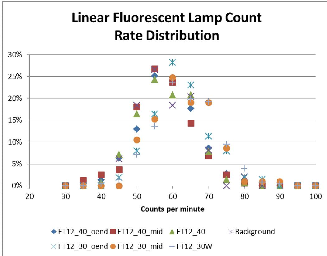
Tests were conducted with conventional “straight” fluorescent tubes, a FT12-30W and a FT12-40W tube at both ends and the near the middle of the tube. The data are indistinguishable from background.
