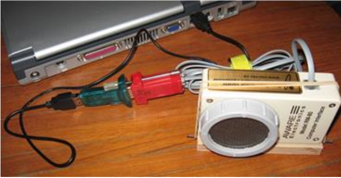
Green USB serial port interface (PL2303) & Red divide by 2 adapter
