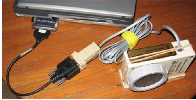
Internal classic serial port (10101) or a PCI interface as shown above with a beige or red cable connector
