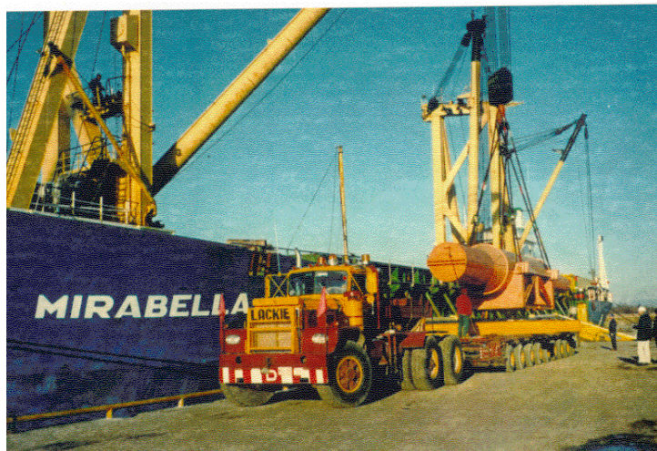
Figure 5.11: Port Hope dock with heavy lift ship unloading a 200 tonne generator rotor onto transfer truck
