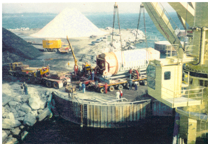
Figure 5.9: Blue Circle dock with heavy lift ship unloading a 350 tonne generator stator
