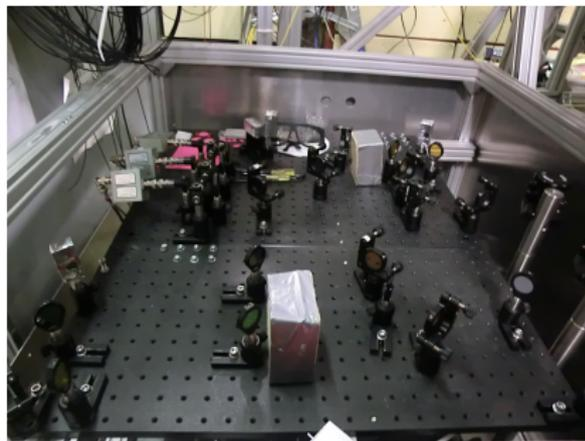
Figure: Polarimeter at GF: (Left) bottom level, (Right) top level.
