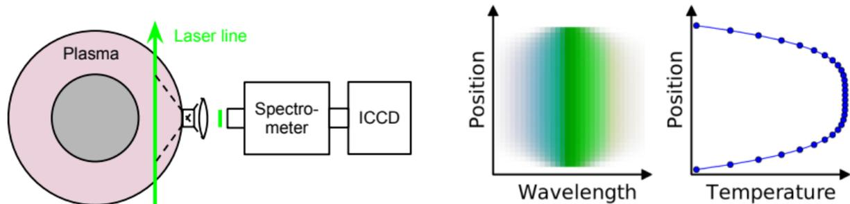
Figure: (Left) 1D Thomson setup. (Right) Simulated 1D Thomson data.
