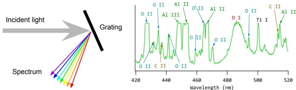
Figure: (Left) Spectrometer illustration. (Right) Segment of visible spectrum measured with spectrometer/camera (by J. McCone)
