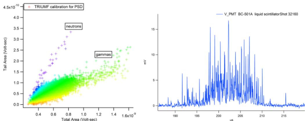
Figure: (Left) Pulse-shape discrimination. (Right) Scintillator detects neutrons.
