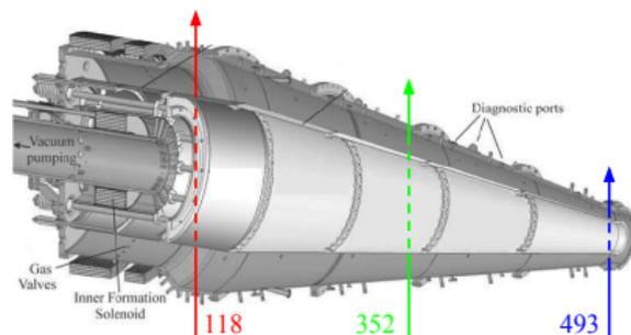
Figure: (Left) Interferometers show plasma being compressed as it travels down injector. (Right) Interferometer positions.
