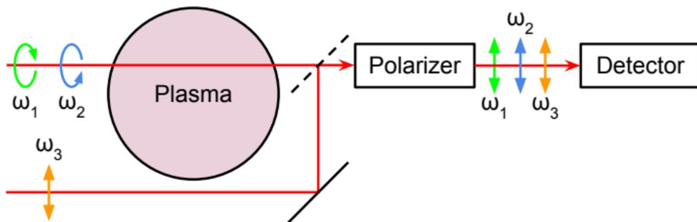
Figure: Three-beam heterodyne polarimeter.
