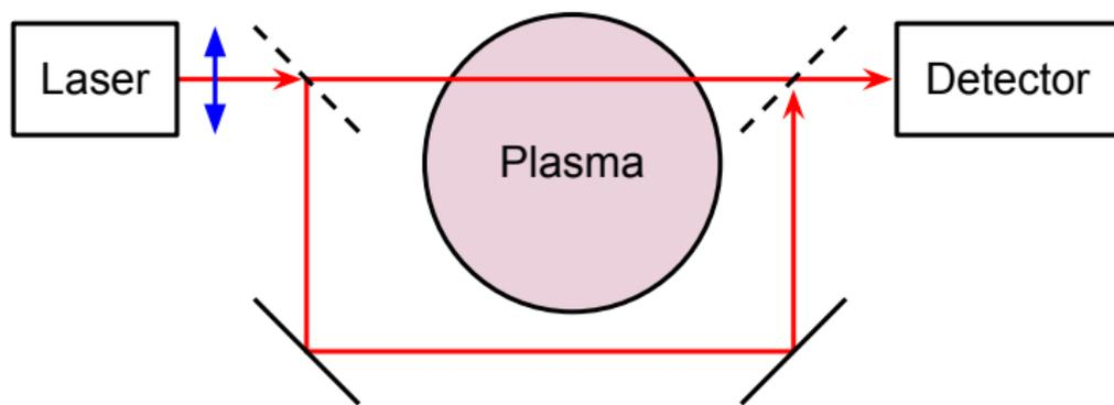
Figure: Mach-Zehnder interferometer.
