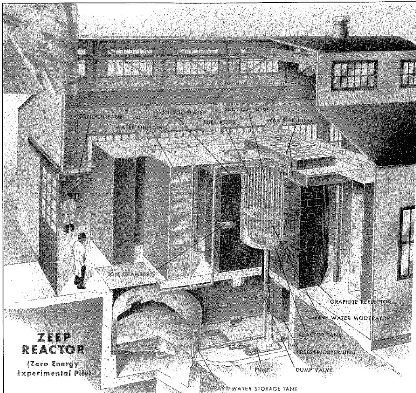
A schematic drawing of ZEEP.
