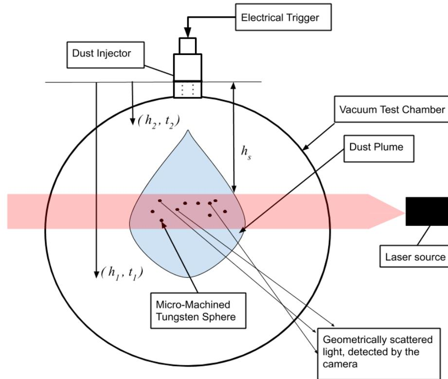
**Data Acquisition Scheme for Dust Injector Calibration**
