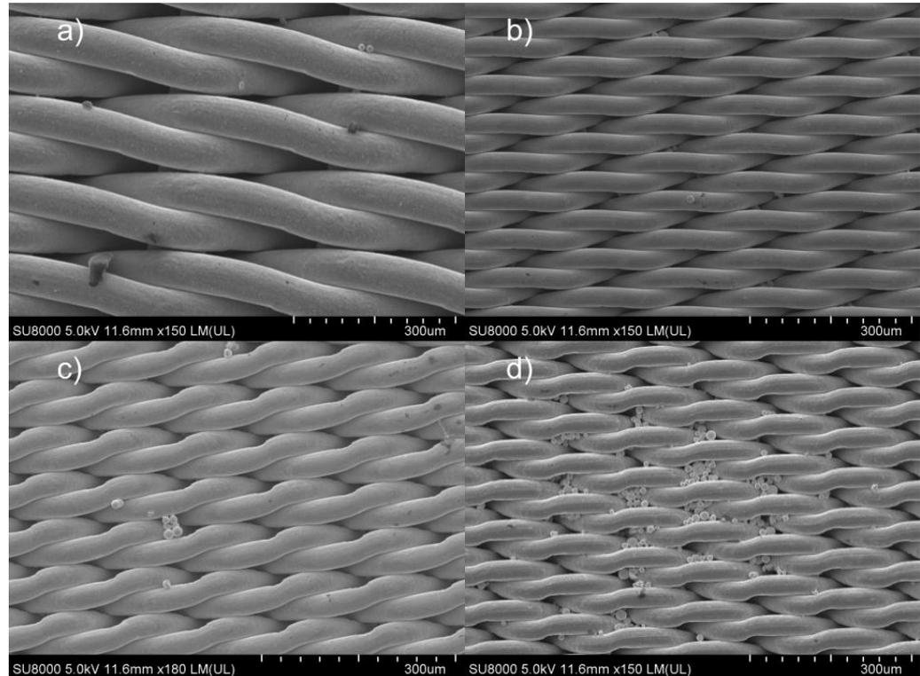
**Dust injector screens imaged with the Hitachi SU8010, FE-SEM at the University of Saskatchewan (After Use)**
