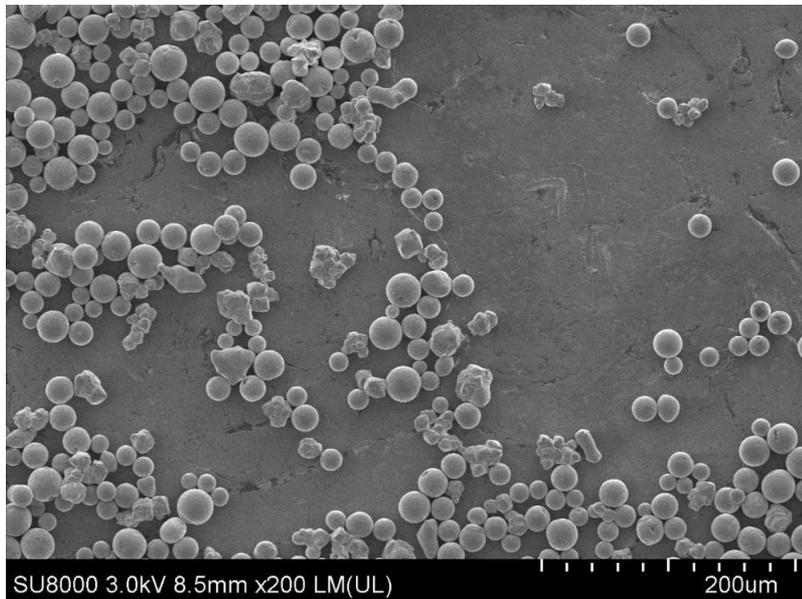
**Spherical tungsten micro-powder imaged with the Hitachi SU8010, FE-SEM at the University of Saskatchewan (Produced by Tekna Plasma Systems)**
