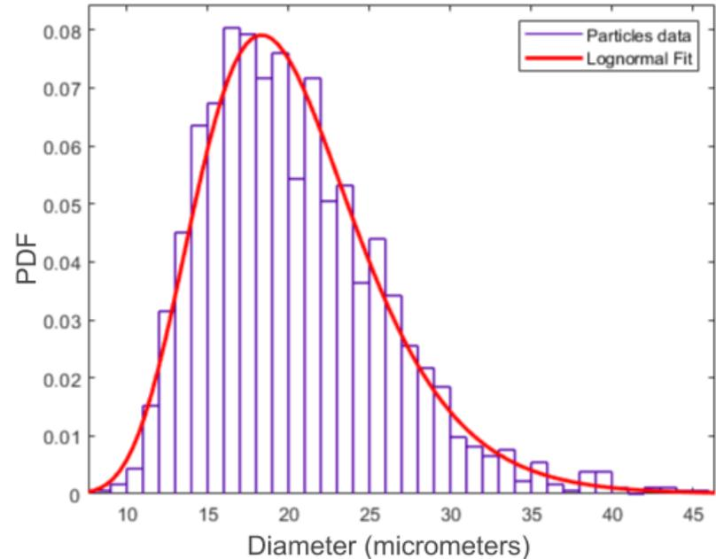
**Probability distribution of spherical micro-particle sizes.**
