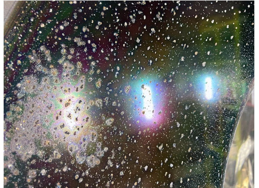
Quartz sample after plasma-facing operation in Helion's 6 th -generation prototype, Trenta.
